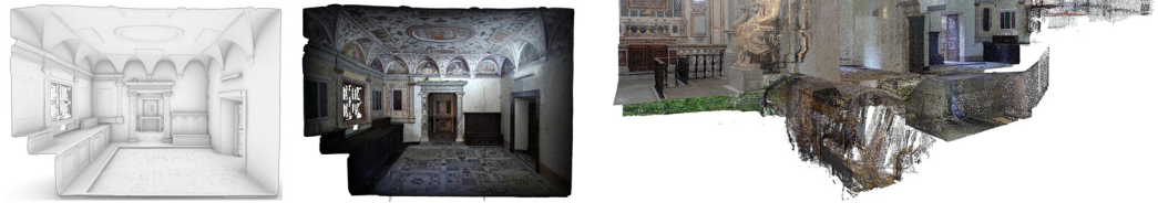
Fig. 11. Perspective view, from point cloud, of the Church of San Pietro in Vincoli, sectioned on the old sacristy. Some clouds have been hidden to highlight the tomb of Julius II and the rooms of the sacristy (Author's elaboration).
