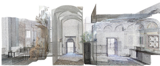
Fig. 10. Section of the cloud of points that highlights the Moses / antisacristy / sacristy sequence of the node to be surveyed. Mesh restitution of the old sacristy in gray scale, to appreciate the shapes, and a render that highlights the cycle of frescoes and the Cosmatesque flooring (Author's elaboration).
